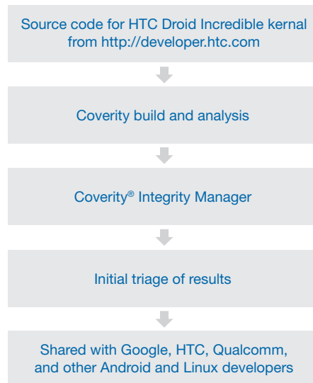
Figure 2: The Android kernel code testing process
